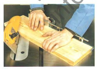
Compound angle With a canting main blade, and accurate mitre fence usually difficult compound angles can be produced easily.
